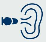
The earplug must be inserted well inside the ear canal to be effective. Once a roll-down foam earplug is prepared, quick insertion is a key to getting adequate attenuation.
